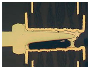
Large void in solder of a plated-through hole connection. 50 x
